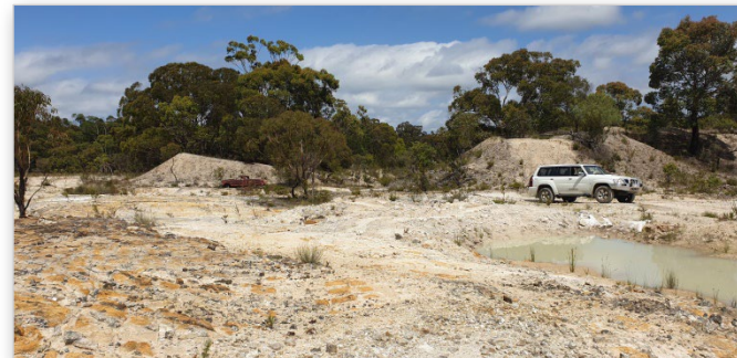
Lode Creek overburden mullock dumps (200kt) carrying tin and wolframite (tungsten) overlying greisen altered granite.
