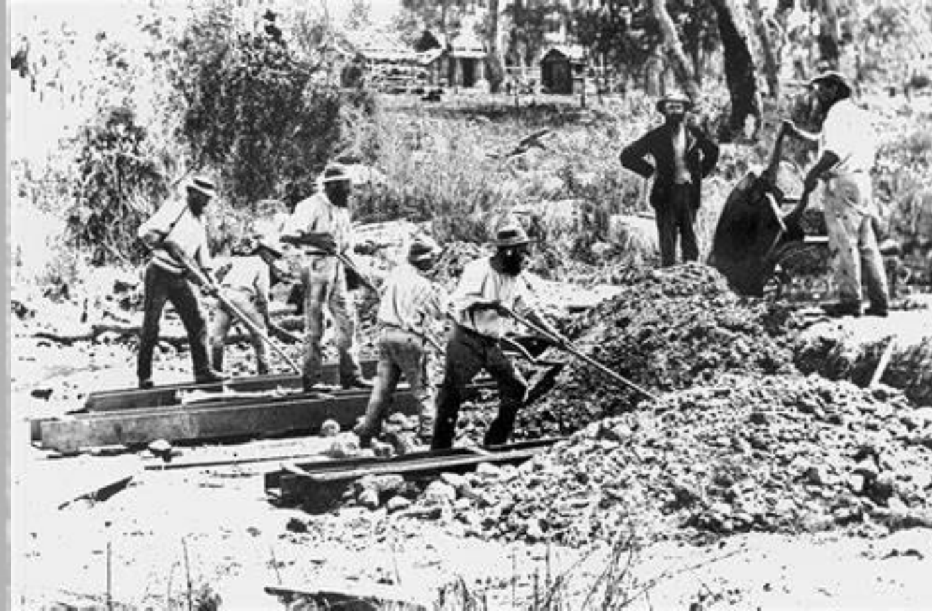
Sluicing with "long toms" at Quart Pot Creek & Funkers Gap on the range
