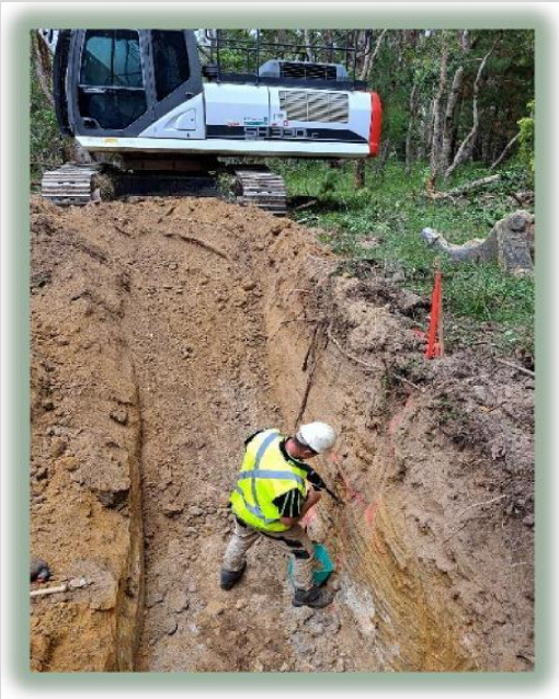
Channel sampling in alluvial bulk pits
