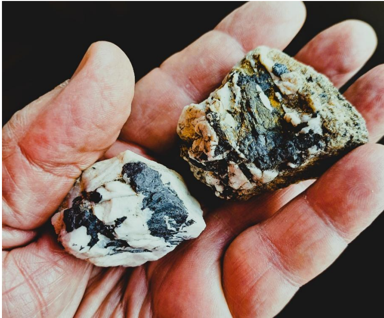
Fig 8 Wolframite (tungsten) within quartz recovered from the overburden dumps at Lode Creek
