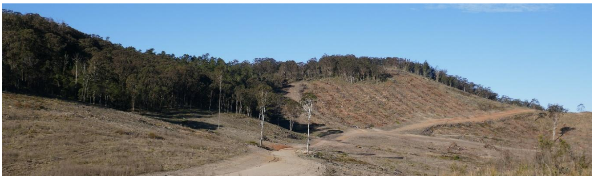
Fig. 1 View looking southeast towards Mt Sugarloaf (one kilometre distant). The NSW border is on the far treeline. All the cleared ground in the photo is geologically the greisen rich granite zone with numerous aplitic intrusions. The greisen zone is characterised by quartz vein stockworks which are mineralised with principally wolframite (tungsten WO 3 76.5% and cassiterite (tin SnO 2 75%– 78% ) and minor bismuth, molybdenum and other critical minerals.
