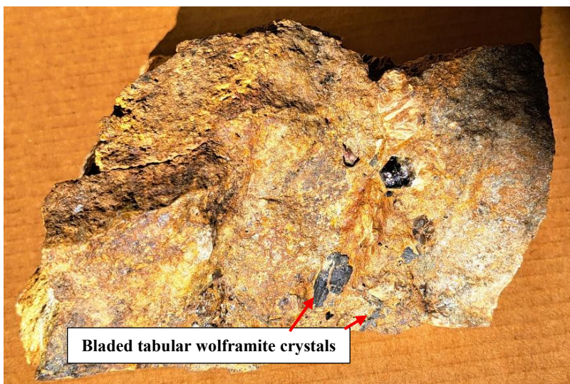
Fig 7 Specimen showing bladed crystalline wolframite (tungsten) and Cassiterite (tin) in the greisen quartz vein contact zone.
